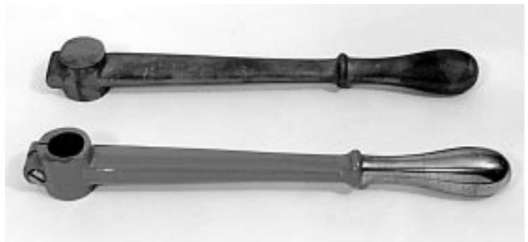
5. Casting made for replacement handle (above) and after machining and painting (below).
