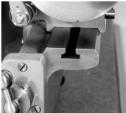
4. The substantial bed-section of the American Watch Tool Company milling machine (40mm across flats).
