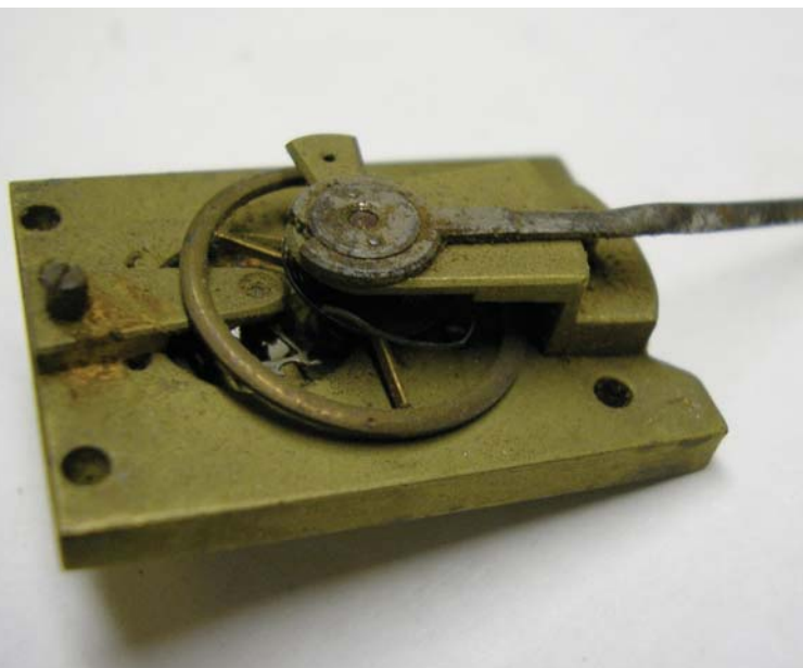
1: Cylinder platform beyond economic repair.
