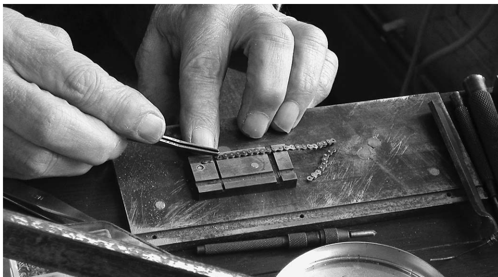
14. Assembling the links in the groove in the assembly tool.
