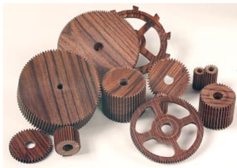
3. Some of the train wheels. The great wheels (solid) and broad pinions of the train. Note the 10-tooth escape wheel.
