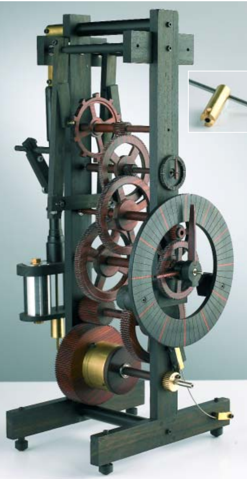
1. Sculptural table clock with ebony frame and dial with wheels, arbors and pinions in Indian rosewood. Many of the arbors run in ball races. These are also used for the pallets in the unusual 'swing escapement' in which the pallet arms are fixed to an articulated trapezoid frame (see also, 5). At 45cm in height the clock has 'a presence' in a room. Note the unusual winding key, inset, engages the screw head on the ratchet wheel.
