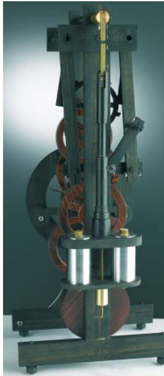
5. Rear view of the clock showing the arms of the swing escapement and the crutch, which bears on the turned ebony pendulum rod via a ball race.
