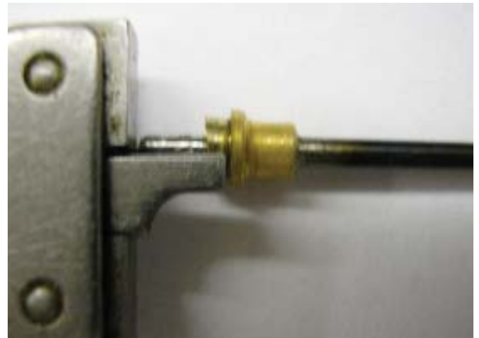
Figure no 5: Measuring original collet seat distance with vernier gauge
