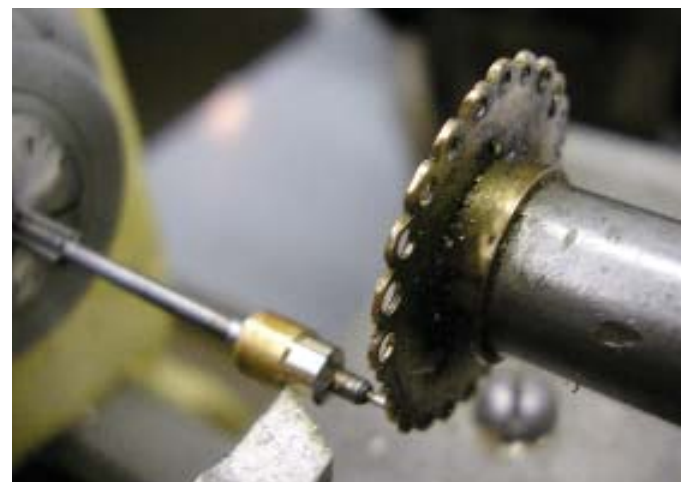
Figure no 6: Wheel seat turning set-up
