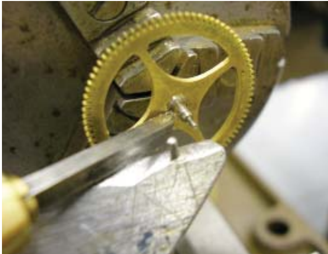
Figure no 3: Removing the rivet
