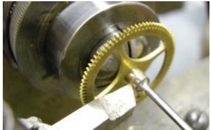
Figure no 8: Set-up for turning collet to shape
