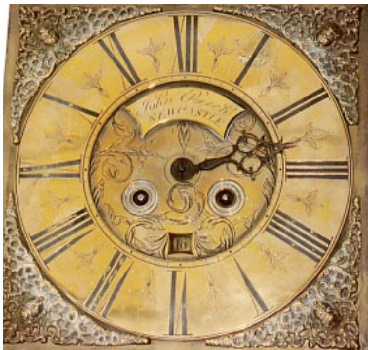
2. The eleven-inch square brass dial of the John Beech clock, looking for all the world like an eight-day single-hander.
