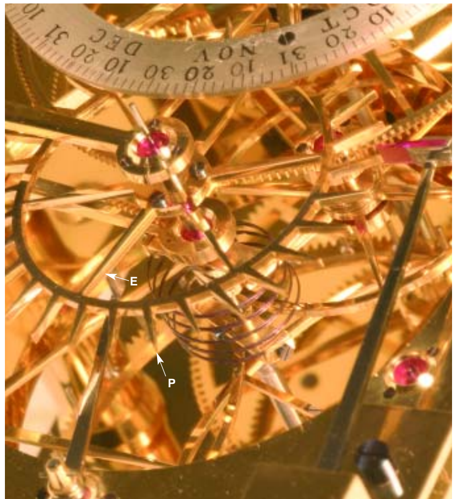
4. Detail of the escapement viewed from below. The arbor of the pin-wheel, P (see also 3) is aligned with that of the escape wheel to which it is linked by the spiral spring. This assembly provides dead seconds although the movements impulse on alternate beats of the pendulums.
