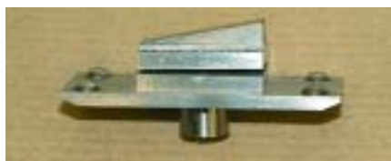
7. This wedge assembly can be raised and lowered beneath the pendulum stirrups lifting the knife edges and clamping the pendulums if required. The spheres and sockets ( 6 ) ensure that the knife edges are correctly aligned when brought back into use.
