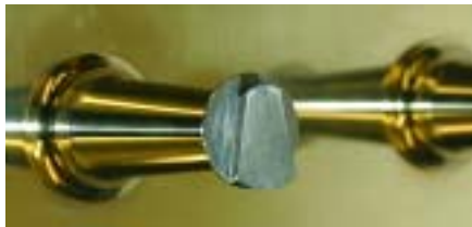
9. One of the movement support pillars on the back plate. The dove-tailed wedges are clamped into sockets on the back of the movements.
