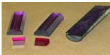
8. Jewels are cut from a synthetic sapphire boule (right). Centre and left are the support jewels and end stops for the knife edge support platform.
