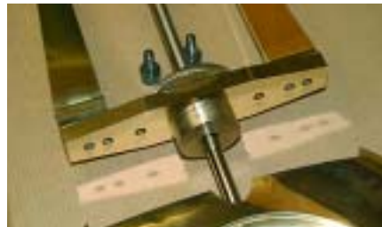
5. Detail of some of the upper and lower components of one of the brass and steel grid-iron pendulums.
