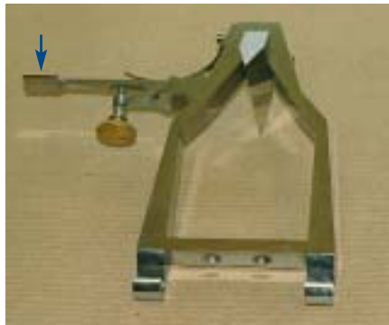
6. The polished steel pendulum suspension stirrup with its hardened steel knife edge and adjustable lateral ruby pallet (arrow) to receive impulse.
