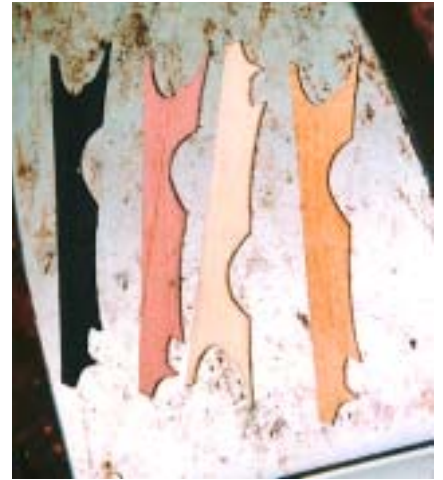
4. A set of identical pieces of the 4 different veneers being dried on a domestic iron.
