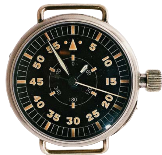
A later Lange & Söhne Luftwaffe hour angle watch, gilt three-quarter plate movement, base cal. 43, in a silver case, marked 92665. Luminous hands for degrees, minutes and radial four-degree indication.
