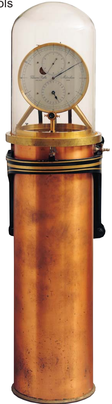
High Command. Regulators such as this one by Riefler, no. 368, defined the standard time, disseminated by the Observatory, and used for rating military chronometers.
