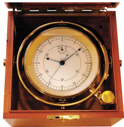
A Lange & Söhne no. 650; an early timing instrument for the German Airforce, four-pillar movement, with hour angle dial, and an external safety hand-setting device. Supplied as a surface chronometer for airfields.
