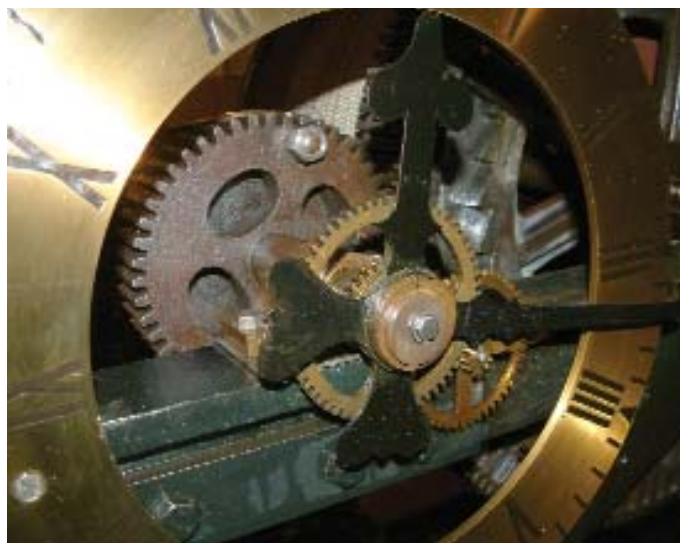
12. A rarely-seen view. The internal setting dial at the rear of the clock. The nut on the gear wheel is one of the two that clamp up the hand setting mechanism.
