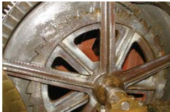
6. The end of going barrel. Note the key that is one of three that retain the great wheel on its arbor. Ratchet-like teeth on the side of the wheel are part of the very effective maintaining power system unique to the Great Clock
