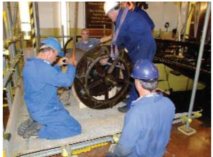
16. Safely in its cradle, the great wheel and arbor is removed from the hour the striking barrel.
