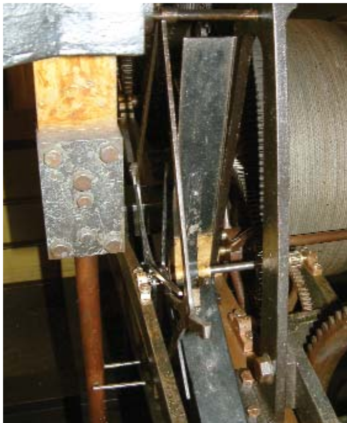
5. The escapement. The Westminster clock is somewhat unusual since it has a three-bladed fly on the 'scape wheel.
