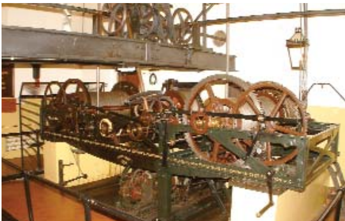
1. The Great Clock Movement: Striking train on the left, going in the centre and quarter striking on the right. The vertical flies are out of view above the movement.
