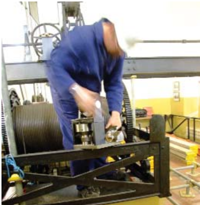
14. Huw removing the safety brake. In the event of over speeding, the brake operates, clamping the great wheel between two brake pads.
