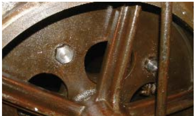
3. Rear view of the hour striking barrel. The bolt heads that secure the cam wheel onto the barrel cap were found to be rubbing on the great wheel. As a temporary measure, the bolt heads were reduced slightly.
