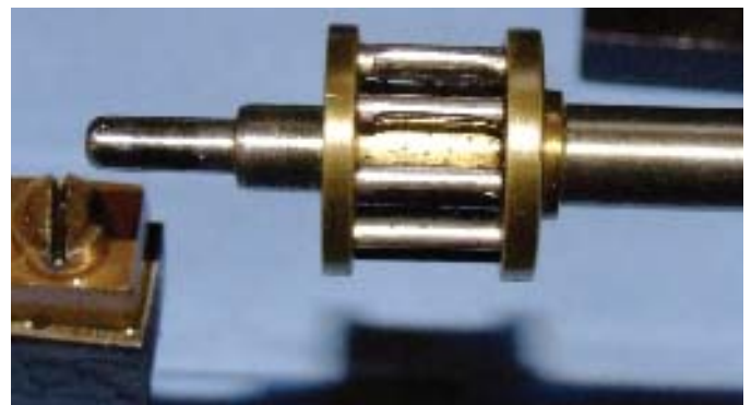
4. Escape wheel pinion, note the wear on the trundles.
