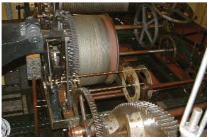
2. Top view of the movement. At the back the quarter barrel can just be seen. In the centre is the going barrel with its train and escapement. Note the two wheels on the going barrel, the great wheel on the left, the right one is a winding wheel on the barrel itself. In the foreground the cams of the hour striking barrel can be seen along with one wheel of the striking train.
