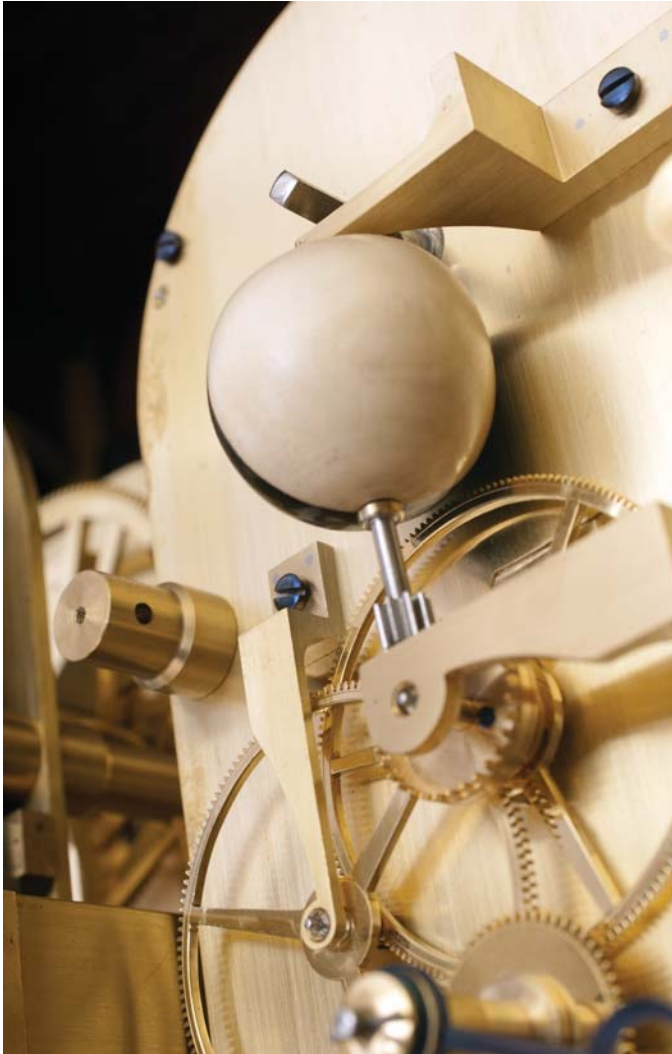
Contrate drive for the spherical moon which is made of ebony and holly.
