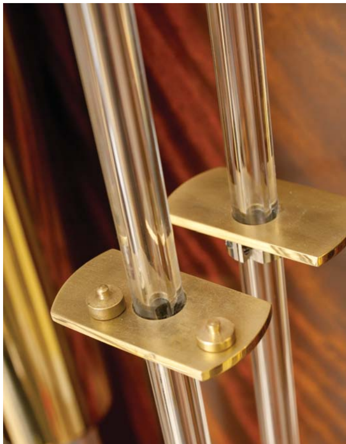
Weight trays on each pendulum, the collars holding the matted brass trays are Invar.
