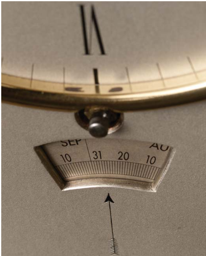
Date aperture in the French silvered mean solar dial, the shaft above the date is for setting the hands using a special key.
