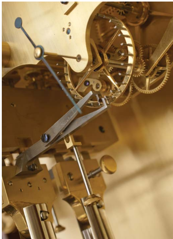
Sidereal movement escapement showing the method for attaching the pallets to the suspension.
