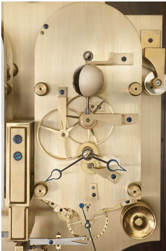
Sidereal movement showing the lunar train.
