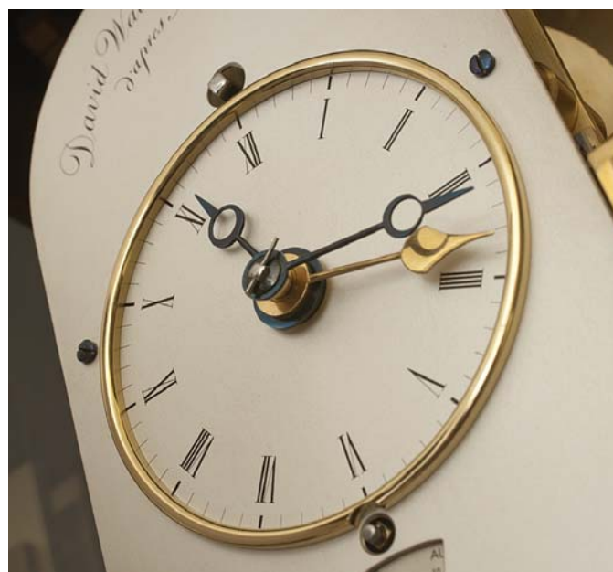
Mean Solar dial with equation of time indicated by the gold hand.
