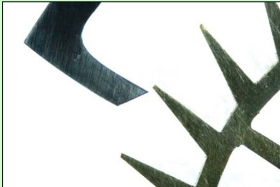
Slightly too large, tooth tip is too thick.
