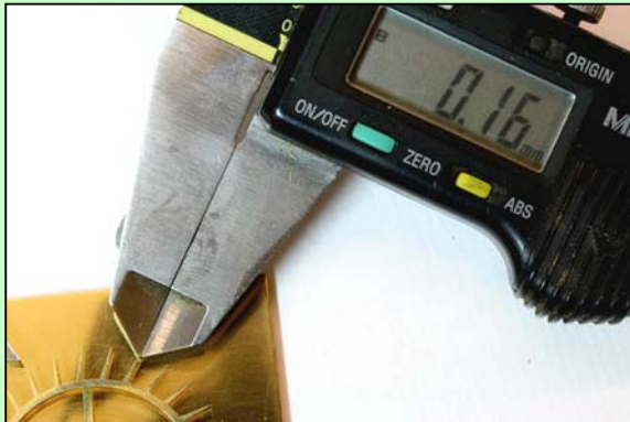
Cut the teeth and check the tip thickness
