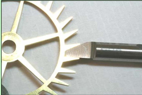
The cutter must match the tooth shape.
