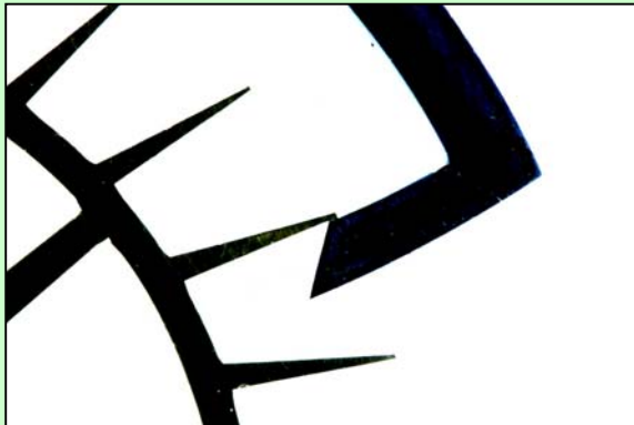
Depth of locking slightly too large.
