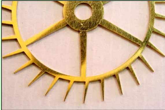
The “rim” is uniform, corners sharp.
