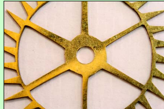
The boss is not circular, corners rounded.
